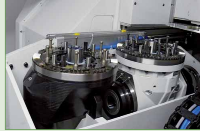
Photo: Spindle attachment pickup station with 6 positions
